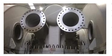
The new turbine has been designed to avoid the remarkable corrosion issues that affected the original one. To withstand the extremely aggressive chemistry of the geothermal fluid from the local basin, the retrofit turbine casing's inner surfaces are made of highly corrosion resistant martensitic stainless steel instead of the carbon steel conventionally used for this type of applications.
