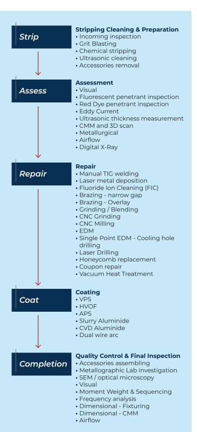
**Repair Innovation:** Coupon repair, selective laser melting, new materials and techniques for repair, extension of life time (multireco) and operating range.
