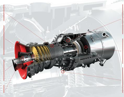
\*All vanes and blades replaceable with rotor in place.
