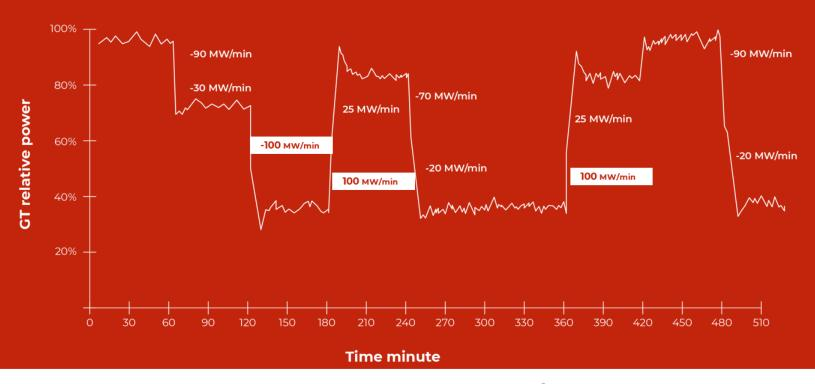
GT36: load gradients of ±100 MW/min in use
