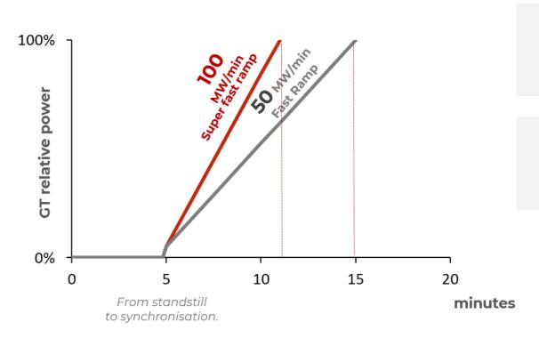
**15 min** to Full load with Fast Ramp rate
