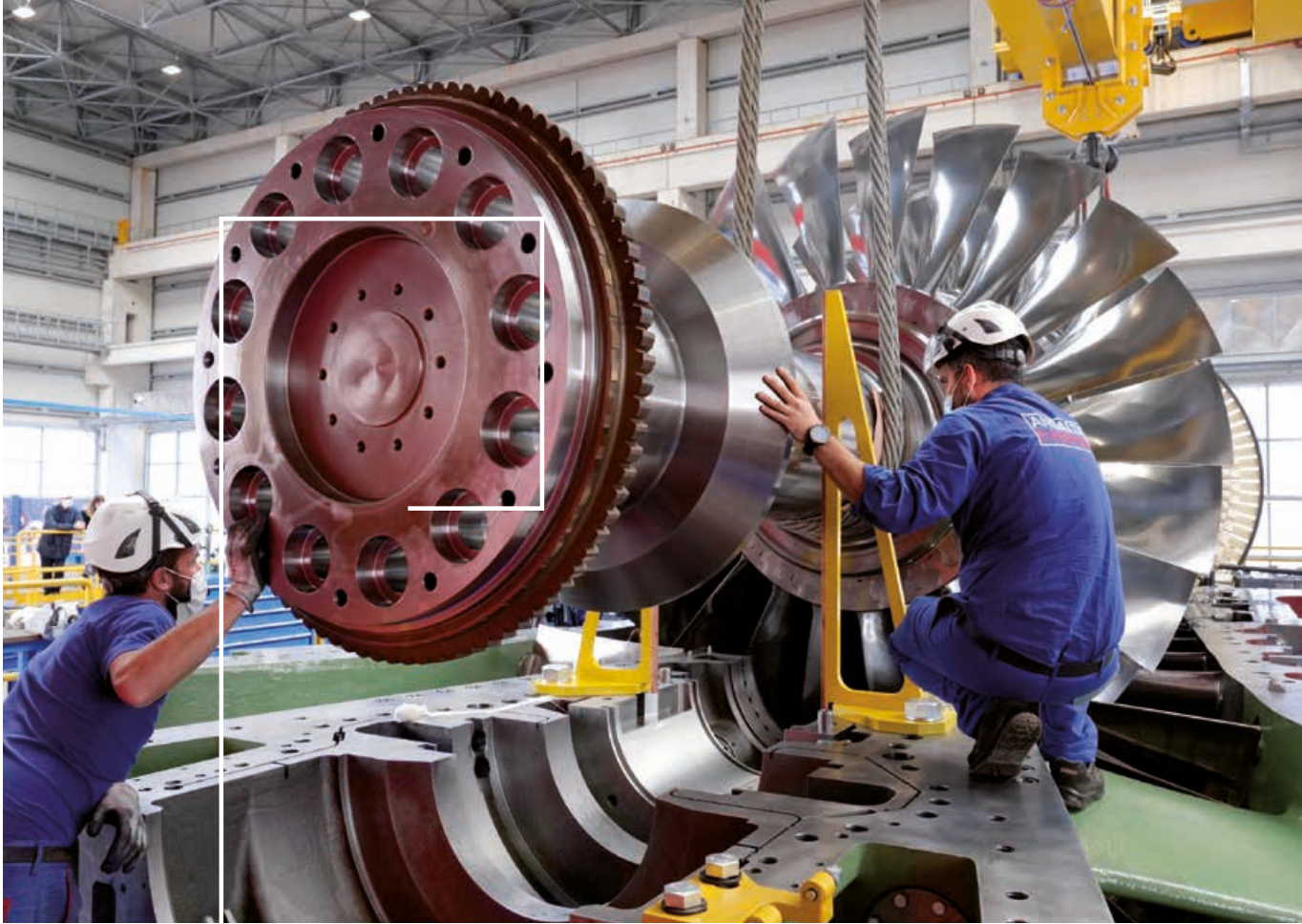
GT36 gas turbine assembly
