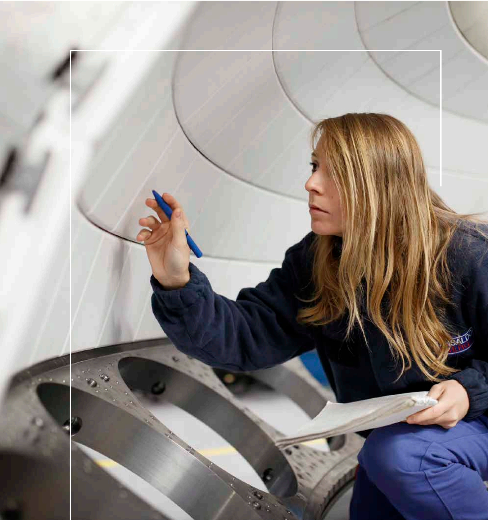
Tile control of a gas turbine combustion chamber
